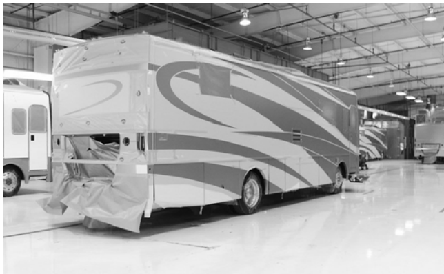
The main color has been applied and baked, and the unit is masked for the next step in the painting process
