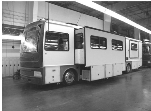
Everything has been installed, and the unit is ready for PDI prior to being painted
