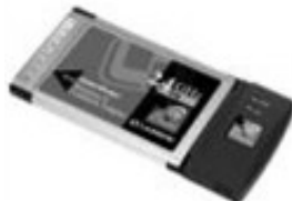
A "wifi" card which is inserted into your computer for wireless Internet access.
