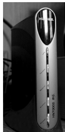
Whether you use a tripod system or a roof mounted dish, the modem from HughesNet will most likely be the HN7000S, using the KU band satellite. Typically, a modem will plug into a router like a home-wired DSL or cable modem, and make the Internet available to your network via wired or wireless connections.
