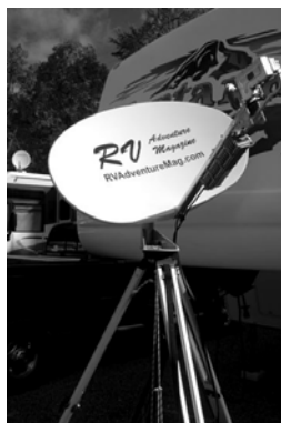
Satellite Internet can be received from a simple tripod mounted antenna. This .74-meter dish has been used from central California, into southern Canada, and east to New York with no trouble. It's been commissioned to the G16 satellite located at 99 degrees west. Photo by Don Fink
